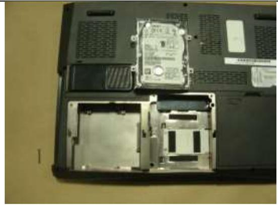
When the hard drive has been removed it should resemble the picture
