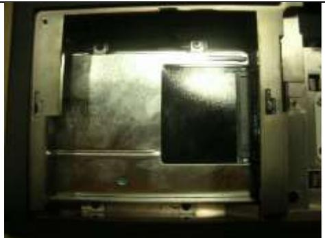
Remove the 4 retainer screws holding the hard drive in place. Slide the hard drive to the left away from the body of the laptop. You will see the gold in color connectors be displayed. Lift the hard drive up and out of the laptop. Make sure not to bind or damage the drive as you remove it.
