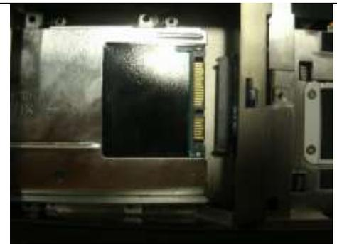
The drive is now removed. Take the hard drive out of the drive carrier tray by removing the side retainer screws.
