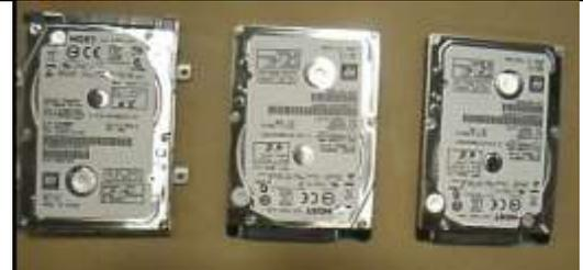
Using the Tableau TD-2 in your kit you will create 2 duplicate or production drives from the master drive. Connect the TD-2 to a power outlet. Turn the TD-2 ON. Let the TD-2 boot up until the Main Menu is accessible. Place the master drive on the left side of the TD-2 and attach it to the TD-2 using the supplied SATA cable. Connect the two production drives to the right side of the TD-2 to Destination 1 and 2 using the supplied cables.
